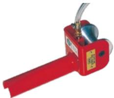
**Duct Entry Guide** (32500 series): This product fits right into the duct opening and has a roller that the cable must pass over. The unit is fitted with a spray nozzle that when hooked up, places the lubricant right onto the cable as it passes under the nozzle.
